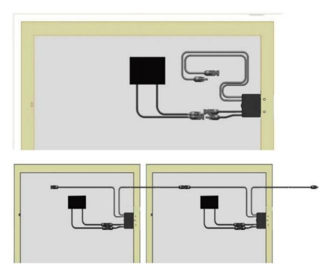
When installing, be sure to connect the input line of the optimizer first, then the output line. When removing, be sure to disconnect the output wire first, then the input wire.
