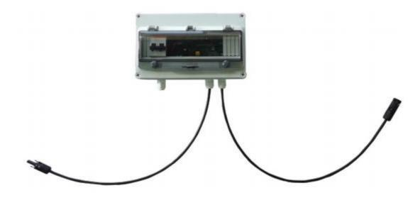
The controller is the equivalent of a control box and gateway integrated into a single string system. The controller has three ports, two of which are pre-installed with photovoltaic cables and connectors (one male and one female), and can be connected in series to a group string.
